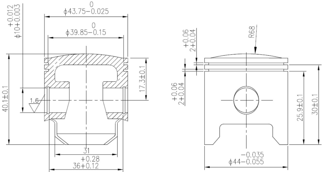
Part No./Factory internal Drawing No.: 1E44F-5.3-1
